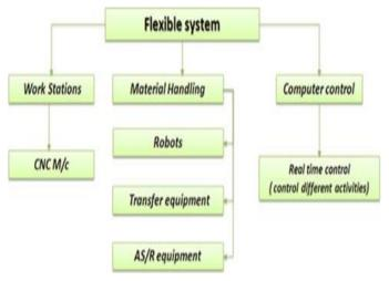
Figure1: Components of FMS
